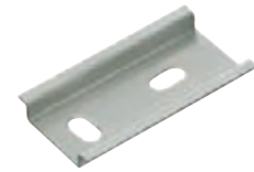
TS 35/7.5 mm according to EN 50022 (s = 1.0 mm)
