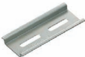
TS 15/5.5 mm according to EN 50045 (s = 1.0 mm)
