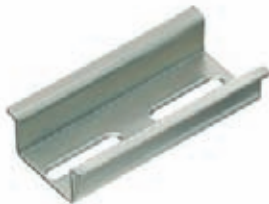
TS 35/15 mm according to EN 50022 (s = 1.5 mm)
