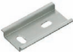
TS 35/7.5 mm according to EN 50022 (s = 1.0 mm)
